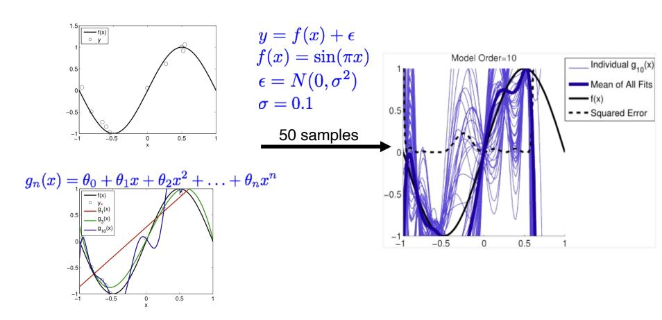
Averaging is a form of regularization: each model can individually overfit but the average is able to overcome the overfitting
